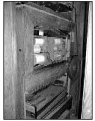
Figure 5. Enclosed in the back of the Wurlitzer 153 are the twin roll frames
